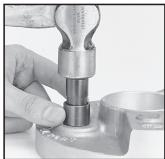
4. Drive keys down with proper installation tool.
