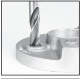
Drill to allow full tap depth shown in chart. Note: Tap drill is oversized; see chart below. Countersink as shown in chart.
