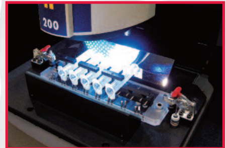
Compact Horizontal Clamps holds syringes in place during processing
