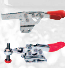
Low Profile in clamped position
