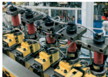
Stamping unit placed in line
