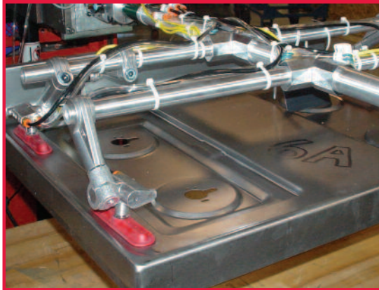
Stove top stamping end of arm tooling using DE-STA-CO Vacuum Products and Round Tooling with Manual Tool Change
