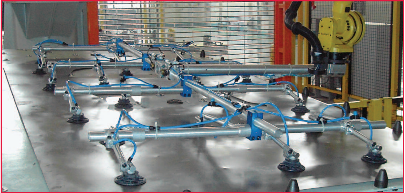
Automotive stamping end of arm tooling using DE-STA-CO Vacuum and World Tool with Manual Tool Changers
