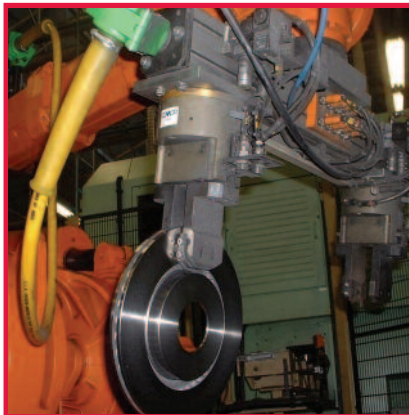
End of Arm Tool using DE-STA-CO Parallel Grippers to pick & place steel tubing and brake rotors
