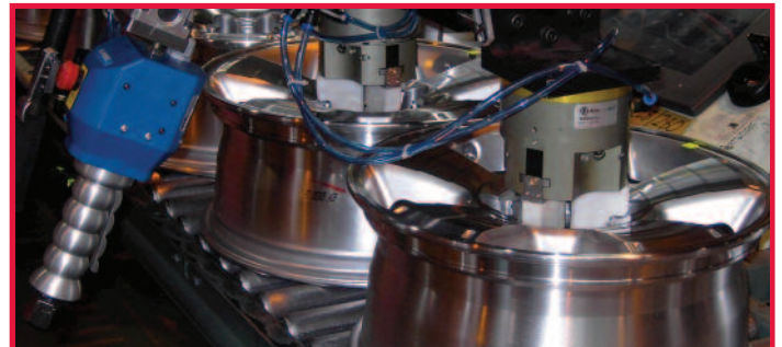
"Below-The-Hook" manual lift assist wheel rim tool using DE-STA-CO Round Tooling and 3-Jaw Grippers
