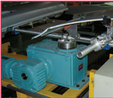
Lower idle stand for press toom transfer using DE-STA-CO Indexers, Vacuum Products and Round framing
